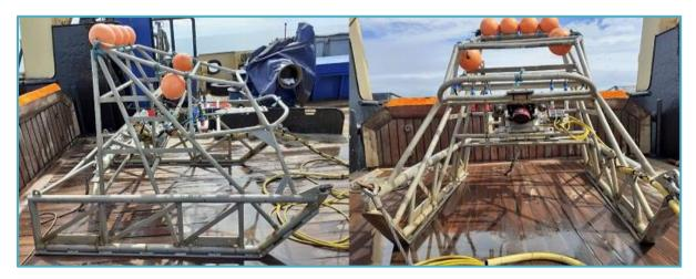
Figure 3: Photographs showing the AFBI camera sledge used during the Summer 2020 surveys.
