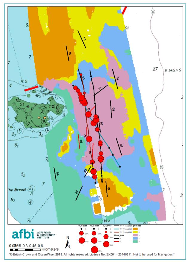
Figure 35: Rox Ann cluster map (from roughness and hardness values) from the AFBI July 2020 survey of The Feathers, overlaid with the dredges undertaken on the 28<sup>th</sup> of July 2020 and the video tows undertaken on the 13<sup>th</sup> of August 2020.
