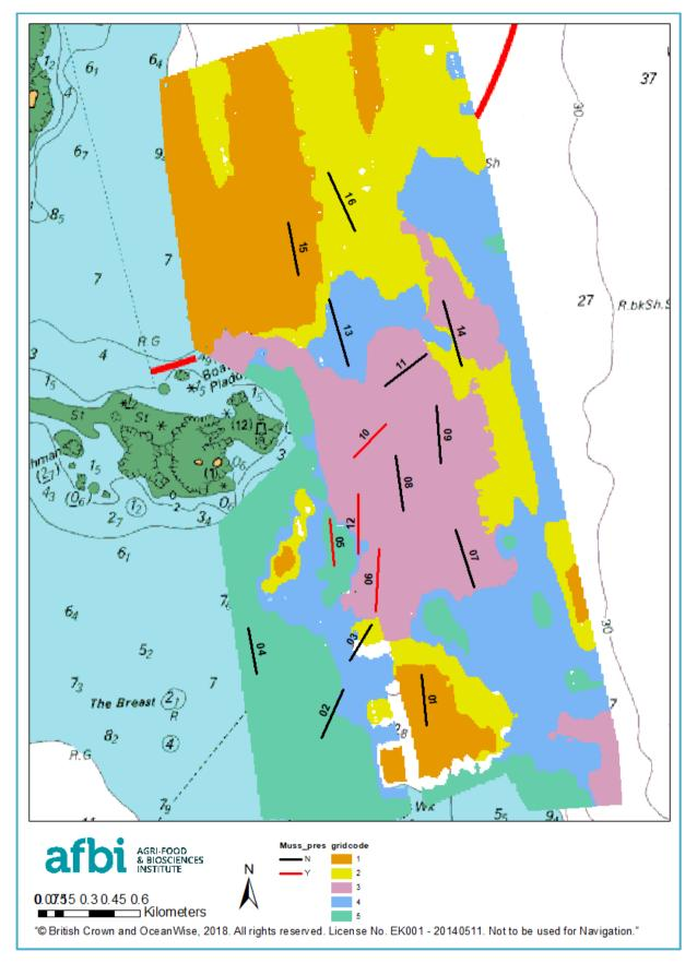
Figure 24: Rox Ann cluster map (from roughness and hardness values) from the July 2020 survey of The Feathers overlaid with the dredge tows undertaken on the 28<sup>th</sup> of July 2020. Dredges within which mussels were found are coloured red.
