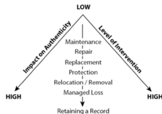
A hierarchy of intervention stages in the life of a building highlighting the importance of basic maintenance in supporting long-term resilience. (Ewan Hyslop, Historic Scotland, pers comm.)
