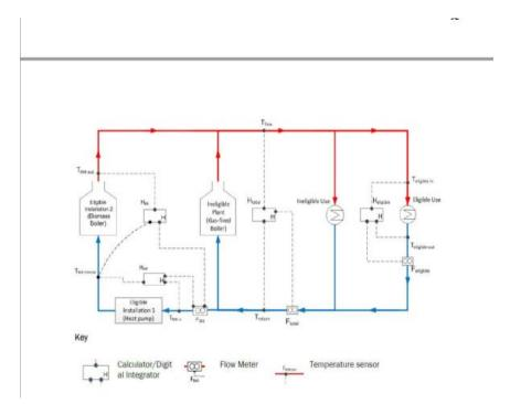
Figure 1.5: Illustration of permissible heat meter locations for a system where a heat pump (eligible installation 1) pre-heats water delivered to a biomass boiler (eligible installation 2).
