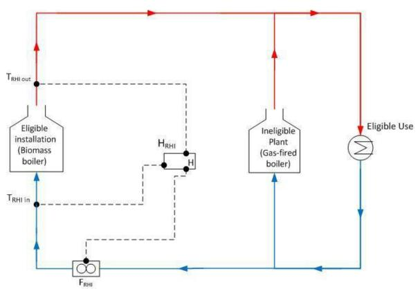
Figure 1.1: Illustration of eligible metering arrangement for a simple installation. The flow meter can be placed in either the flow or return pipe (red lines denote the hot 'flow' pipes, and blue lines indicate the cool 'return' pipes).
