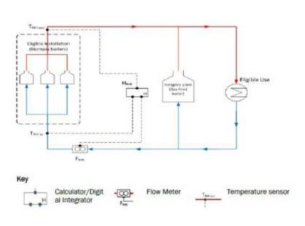
Figure 1.4: Illustrative example of a situation where a shared meter would be permitted. This installation would be classed as 'simple' for NIRHI metering purposes.
