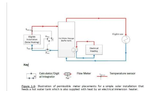
Figure 1.6: Illustration of permissible meter placements for a simple solar installation that feeds a hot water tank which is also supplied with heat by an electrical immersion heater.
