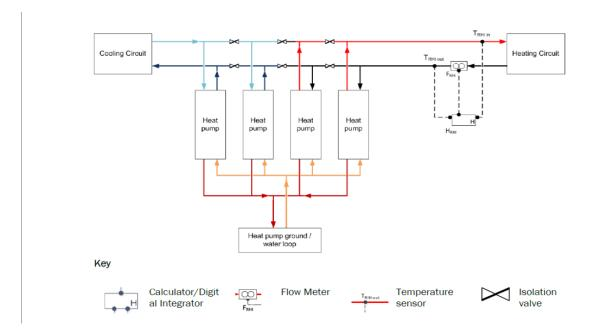
Figure 1.7: Illustration of permissible meter placement for a simple installation where four heat pumps deliver both heating cooling on a sliding header. In this case, two heat pumps are supplying the heating circuit, and the other two are supplying the cooling circuit.
