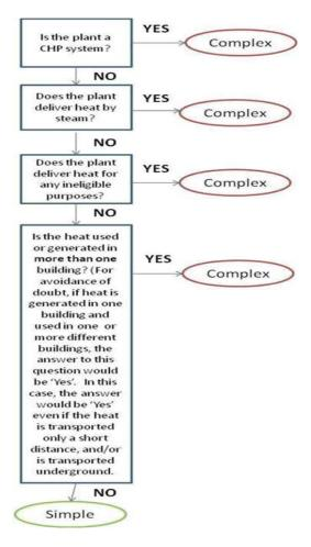
Figure 4: A flow chart illustrating whether a plant comprising all or part of an eligible installation would be classed as 'simple' or 'complex' for NIRHI metering purposes, in accordance with the Regulations. NB: Where an installation is comprised of multiple parts, it will be classed as 'complex' for NIRHI metering purposes where any of its component plants are classed as 'complex'.
