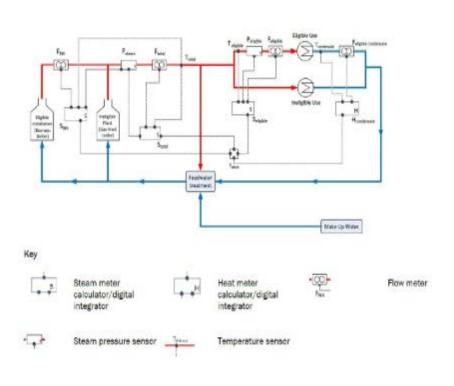
Figure 1.3: Illustration of possible steam meter (and component) placement for a heating system where an eligible biomass boiler and a gas-fired boiler deliver steam that is used for both an eligible and ineligible purpose. Condensate in the form of hot water is returned from the eligible purpose.
