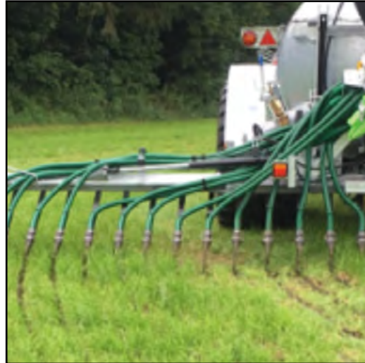
Photo 3 - Trailing shoe spreader
