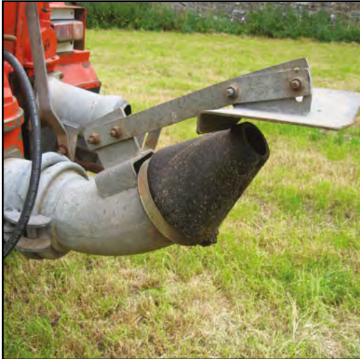
Photo 2 - Inverted splash plate
