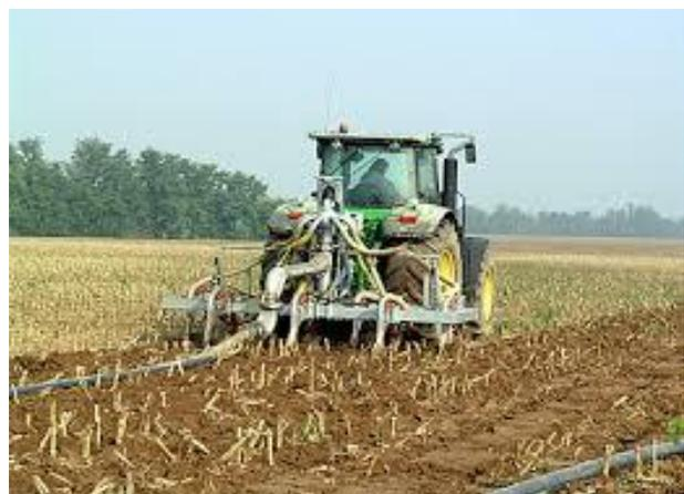
Figure 5 Deep slurry Injection equipment
