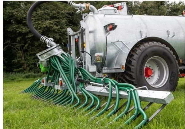
Figure 3b Trailing shoe slurry application.
