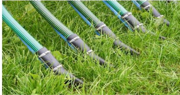
Figure 3a Close up of the trailing shoe parting the grass and the hose delivering the slurry.
