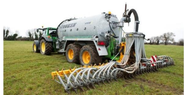
Figure 4 shallow injection equipment
