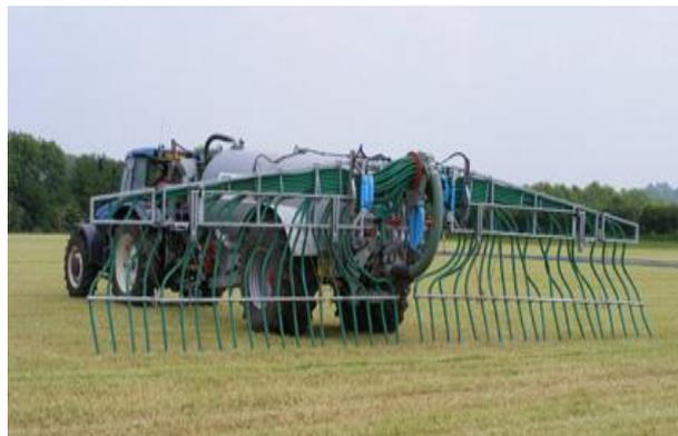
Figure 2a Tanker with trailing hose
