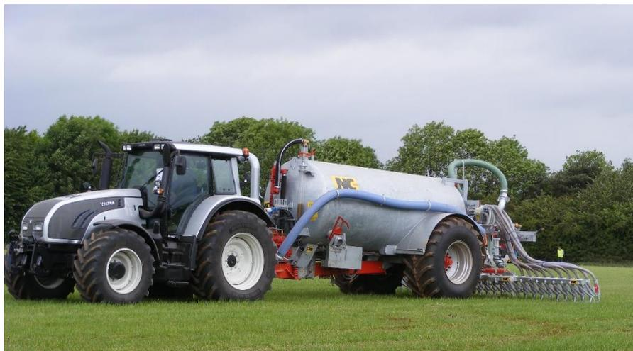
*Figure 1 Slurry application using a trailing shoe system*
