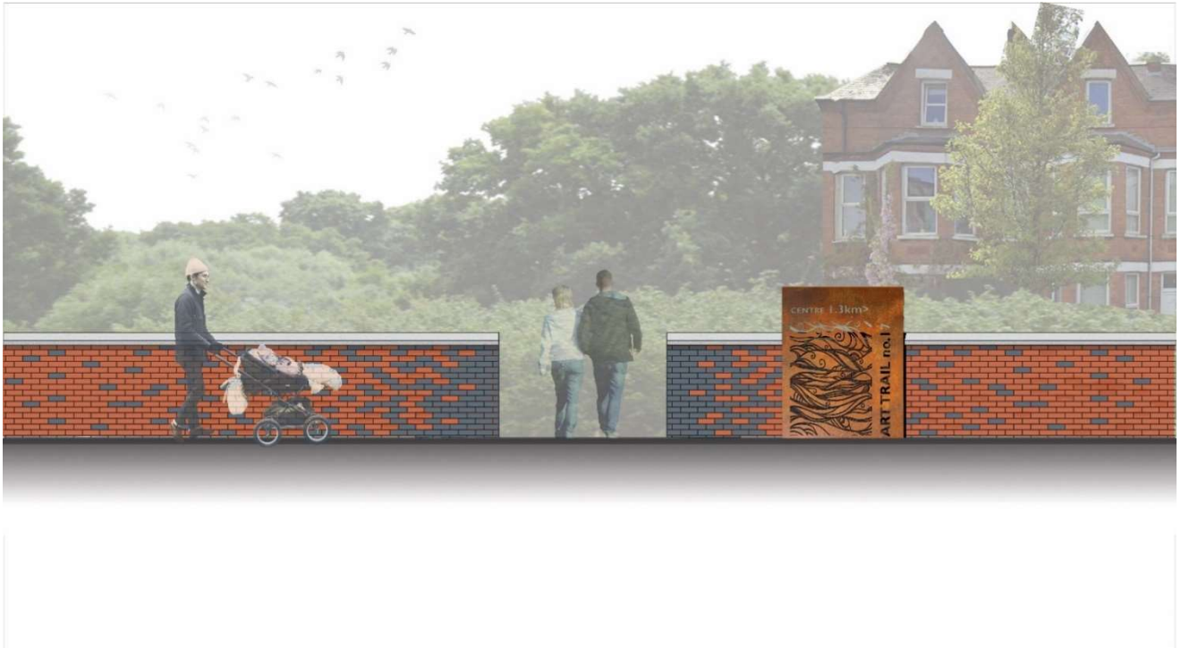
Example of a brick clad floodwall
