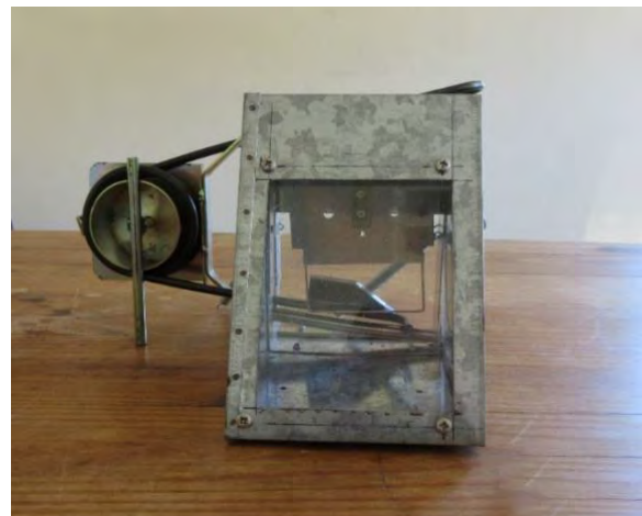
Image 11 - modified Kania 2000 spring trap with Perspex window. © Joe Dowdall
