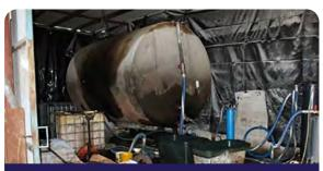
Fuel Laundering Plant where rebated diesel fuel is laundered/washed through 'cat litter' or 'fullers earth clay' material to remove colour from product.
